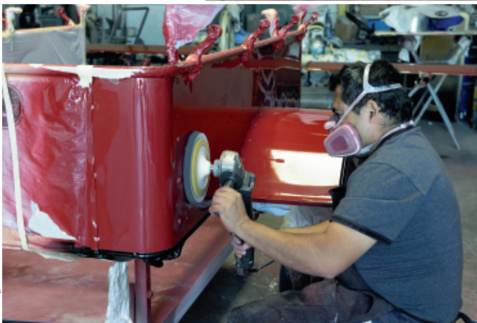
Figure 6 (below) - A paint technician at Tri-Valley Auto Body buffing the newly-painted hose body.
